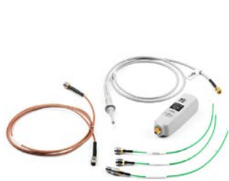
N7020A 2 GHz power rail probe
