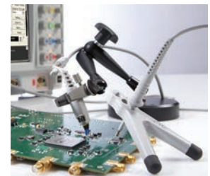
N2786A 2-leg probe positioner and N2787A 3D probe positioner
